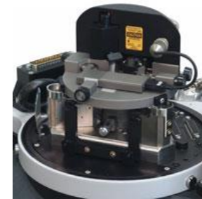
The Configuration for Capacitance Microscopy, Spreading resistance and High Resolution Measurements
