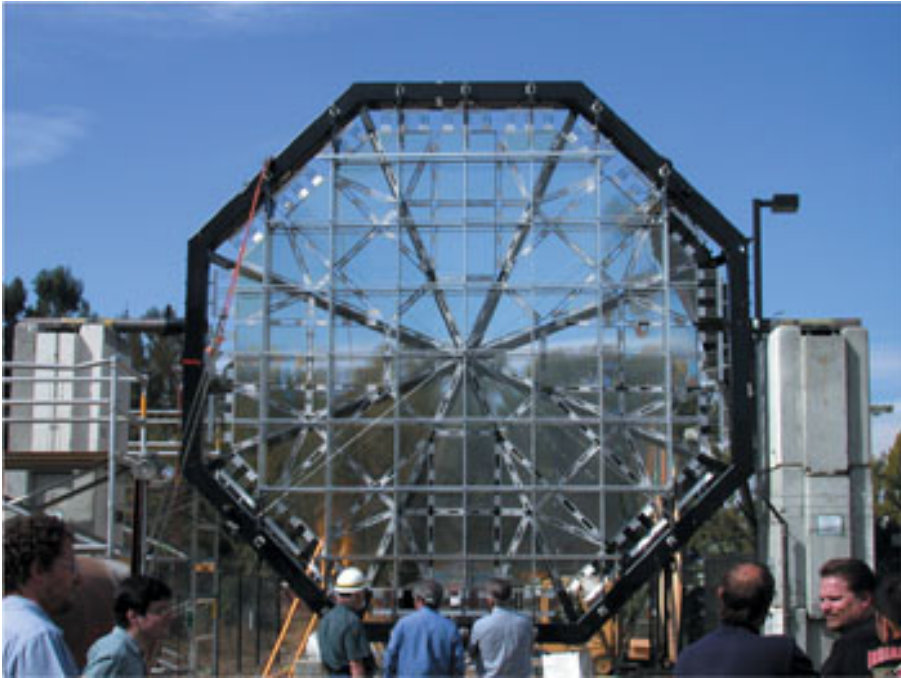
Fig. 12. Picture of a 5 m diameter diffractive lens made by litography (by R. Hyde- S. Dixit).
