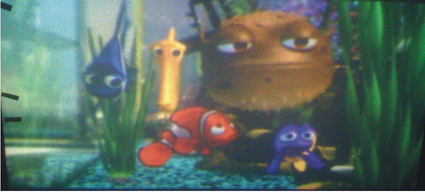
Fig. 8. Projected image at WVGA resolution resulting from a phase-only holographic projection system, employing the techniques described in this chapter, manufactured by Light Blue Optics Ltd. In this instance, \lambda_r = 642 nm, \lambda_g = 532 nm and \lambda_b = 445 nm.
