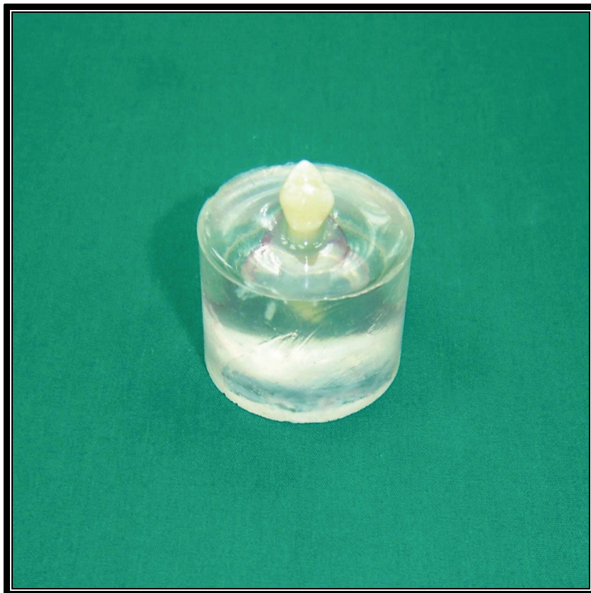
Fig. 1. The tooth embedded in the epoxy resin
