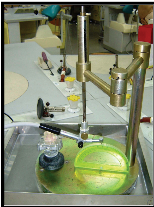
Fig. 2. The paralleling apparatus used
