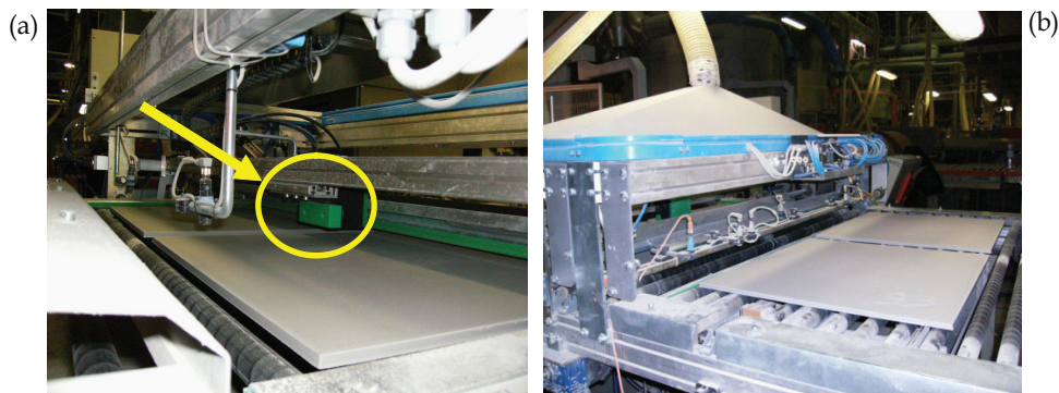
Fig. 8. (a) Head with the sensor holder; (b) Support for on-line positioning
