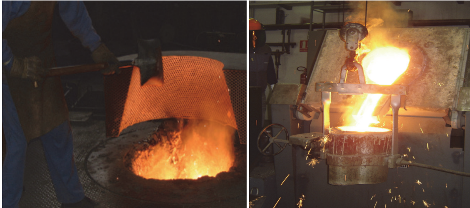
Fig. 11. Masteralloy addition and pouring of steel+carbides
