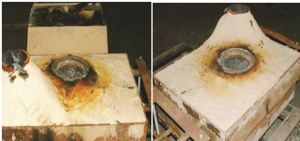
Fig. 13. Mould filled with steel+carbides
