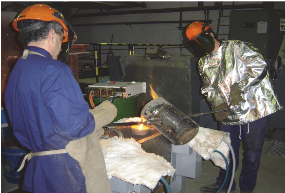
Fig. 12. Mould filling with steel+carbides
