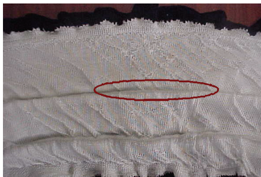
Fig. 37. Preform with jersey evolution on selected needles
