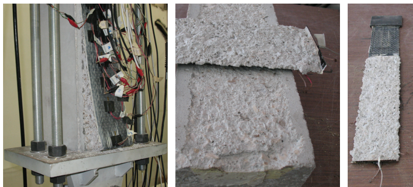
Fig. 11. Specimen after test and typical failure mode
