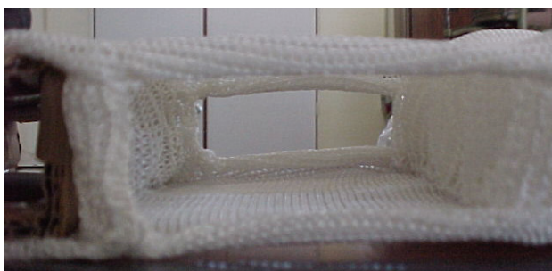
Fig. 24. Sandwich fabric with connecting knitted layers
