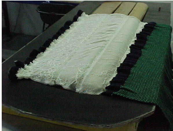
Fig. 44. Introduction of the interior moulds in the preform
