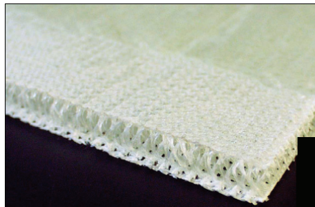
Fig. 22. Spacer fabric made of glass fibre
