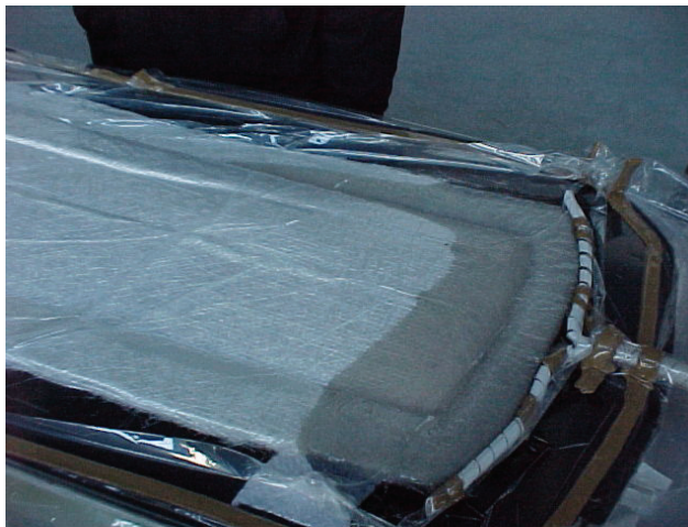
Fig. 45. Resin injection process
