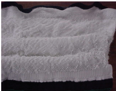
Fig. 38. Preform with jersey evolution on selected needles and fleece in-lays
