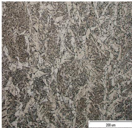
Fig. 2. Typical micrograph structure of acid electrode WMD
