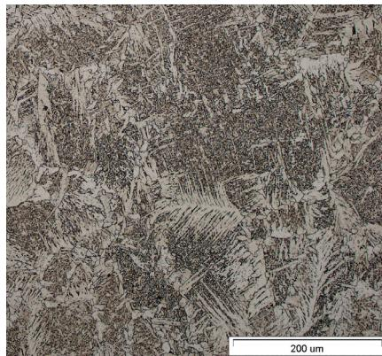
Fig. 3. Typical micrograph structure of rutile electrode WMD
