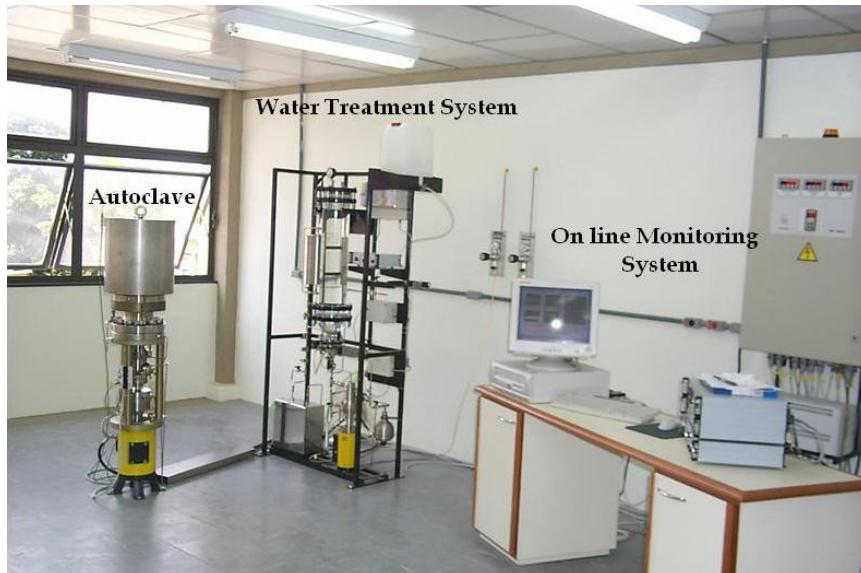
Fig. 8. Photo of the installation of SCC tests.
