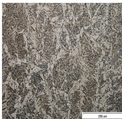
Fig. 2. Typical micrograph structure of acid electrode WMD
