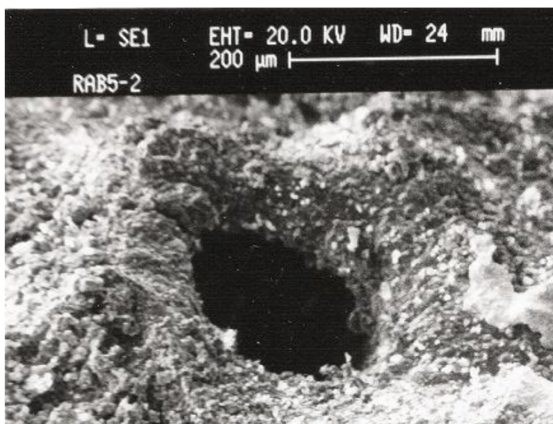
Fig. 1. SEM micrograph of a macropore in sintered bioactive ceramic.
