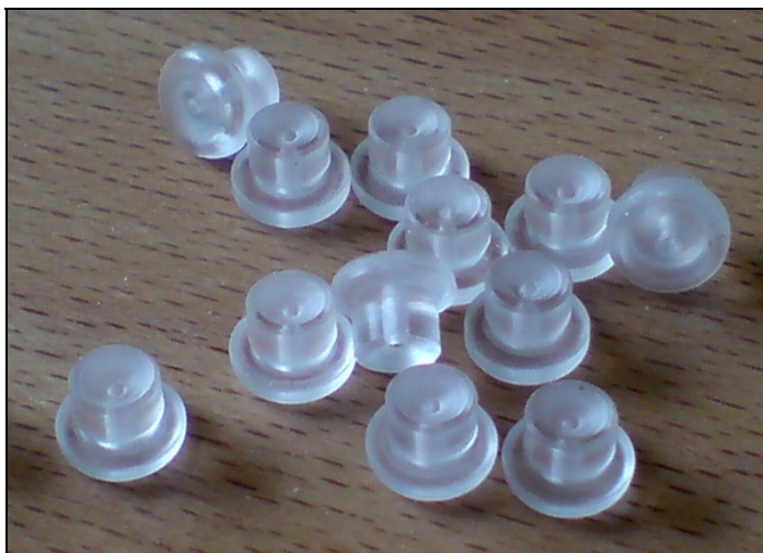
Fig. 2. Poly (2-hydroxyethylmethacrylate) scaffolds – upper parts of hybrid replacements
