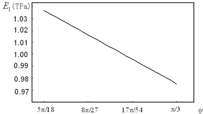
Fig. 12. Elastic modulus of the equivalent model of graphene along the 0^\circ fiber
