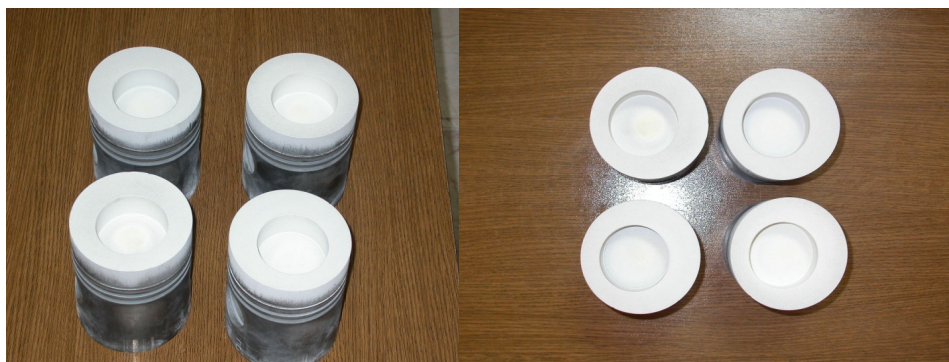
Fig. 10. Ceramic coated piston tops
