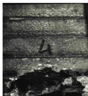
b. mould punching on thicker cross sections of castings
