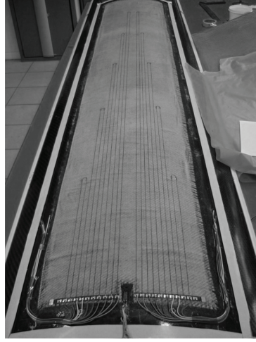
Figure 17. CT tabletop with u-shaped CFSs to measure the deflection. The metallic wiring is attached to the clamping support.
