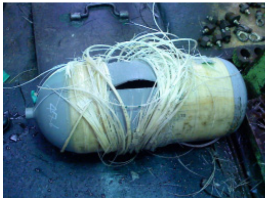
Figure 4. Composite vessel after burst test
