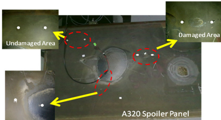
Figure 1. Locations of the structural conditions and PZT sensor placements
