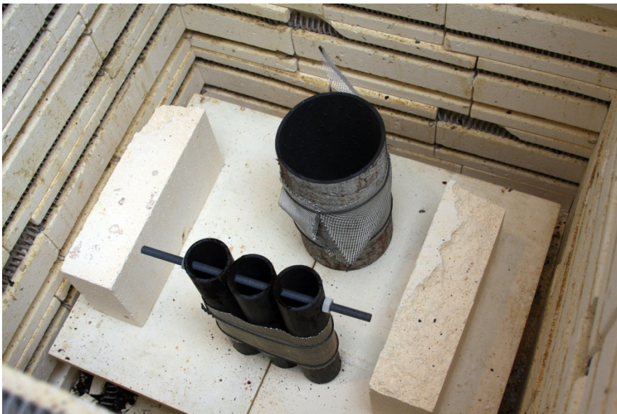
Figure 8. Shape memory alloys and mandrels inside kiln after heating process had finalised.
