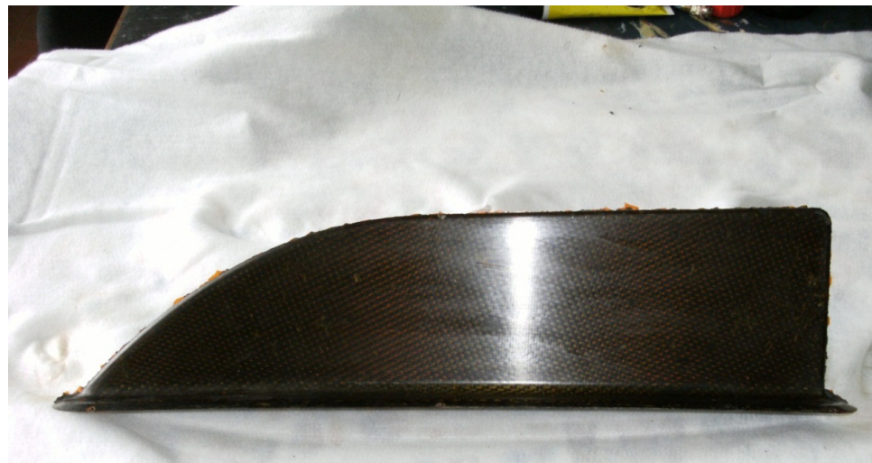
Figure 9. Strake of Aermacchi nacelles after demolding.
