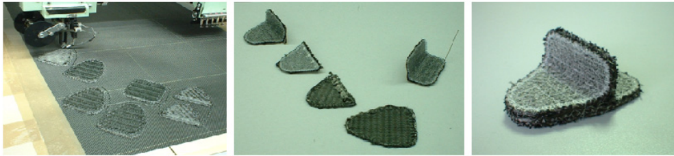
Figure 15. Realization of the preform: cut and stitching.
