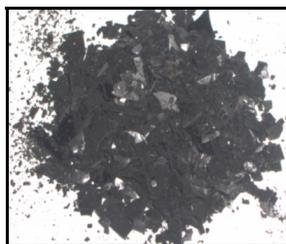
Fig. 6. Illustration of Asphaltenes. Source: Lima, 2008.
