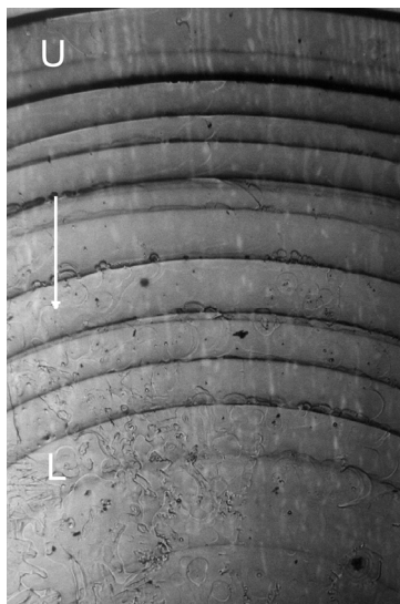
Fig. 4. Micromorphology of a vertical, side (111) surface. U, L-upper and lower parts of a crystal. Arrow indicates direction of gravitational field. Growth temperature: 25 °C. Field of view: 2.7 mm x 4 mm.
