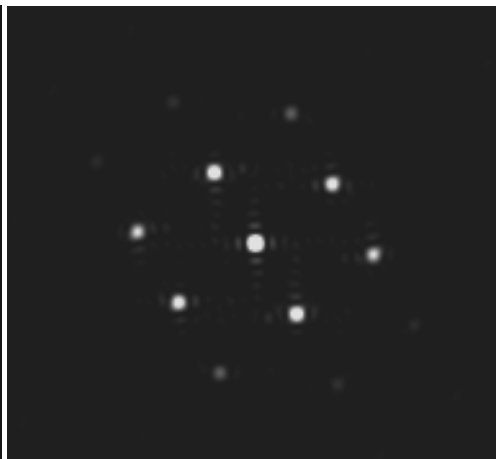
(b) Fourier transform associated to the region delimited by white square in Figure 8c. The distance of the neighbouring central point is 0.58 \mu\text{m}^{-1} in average.
