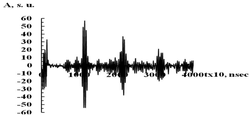
Fig. 2. Oscilloscopegram of impulses with transversal polarization, which are reflected in nanocomposite based on modify teflon-3M and MWCNT.
