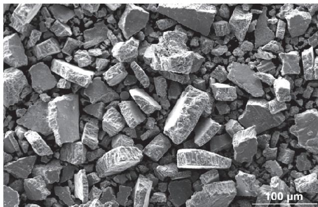
Fig. 1. SEM micrograph taken from ball milled  $\text{Ni}_{48}\text{Mn}_{39.5}\text{Sn}_{10.5}\text{Al}_2$  powders
