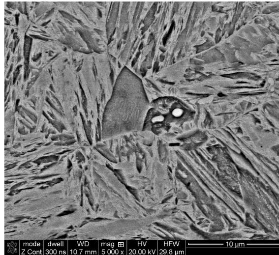
Fig. 1. The microstructure of the investigated steel after  $50\text{ }^{\circ}\text{C/s}$  cooling rate
