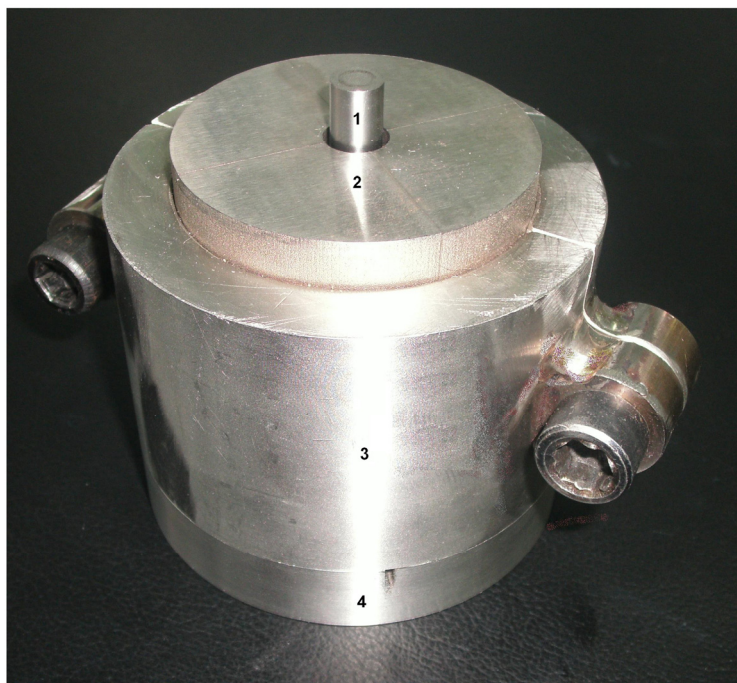
Fig. 2. The four-part dismountable mold is shown in this picture: 1-punch, 2-four-section dismountable block cylinder from high strength tempered steel, 3 - constricting clamp with twotightening bolts, 4 - support with groove for tungsten wire.
