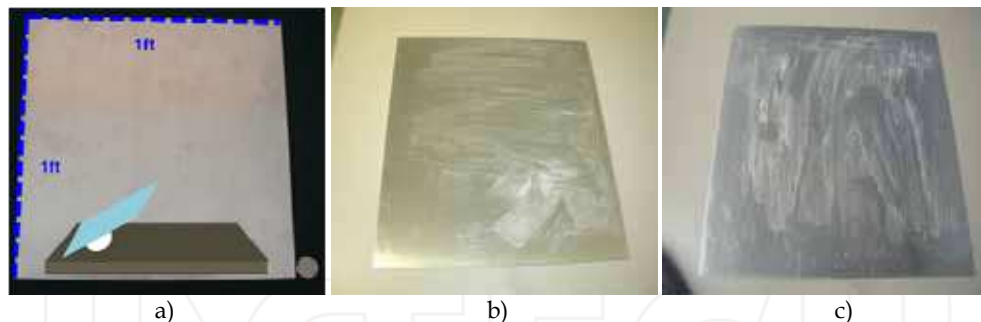
Fig. 2. Sample preparation: (a) Clean Al plate ready for sample smearing technique; (b) 50 \mu\text{g}/\text{cm}^2 of TNT loading concentration; (c) 100 \mu\text{g}/\text{cm}^2 of TNT surface concentration
