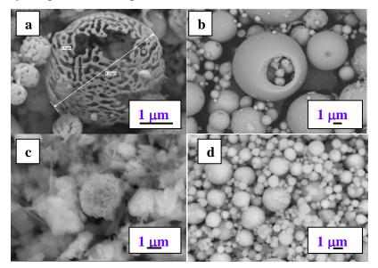
Figure 1. SEM images of powders of alumina and zirconium oxide obtained by spray drying method from solution (a, b) and suspension (c, d).
