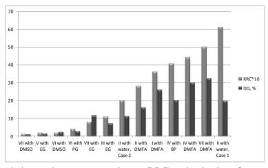
Fig 1. Reflux ratio in entrainer recovery columns (RRC) and reduction of energy consumption by using PCEDS for different mixtures separation.
