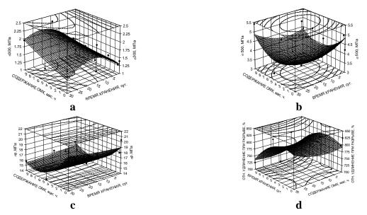
Fig. 1. Dependence of the glue films physico-mechanical properties from the OMC content by the different time of sample holding: a - stress at 300% elongation, b - stress at 500 % elongation, c - tensile strength, d - elongation at break.
