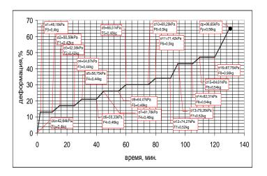
Fig. 2. Creep PE-100 at 100°C and a variable load.
