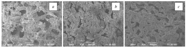
Fig. 1. SEM-images of biocomposite obtained by vacuum impregnation (a), using centrifugation (b), sonication (c).
