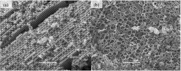
Figure 1. SEM images of macroporous  $ZrO_2$  (a) and  $TiO_2$  (b) samples, prepared by sol-gel synthesis in the presence of PS dried template.
