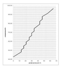
Fig. 3. Dependence of the stress-strain PE-100 at 100°C at variable load.
