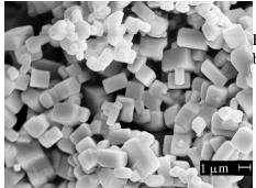
Fig. SEM image of the LLT powder prepared by sol-gel method after sintering at 1000°C.
