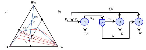
Figure 1. The diagram of phase equilibrium of ternary system IPA – D – W (a) and principal technological separation scheme (b). The material balance lines are shown for case IV.
