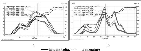
Fig. 1.- Data of dielectrical analysis of the process of curing of epoxy-carbon composite material: a - non-modified, b - modified.
