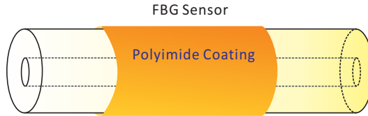
Figure 2. Illustration of a FBG sensor with polyimide coating
