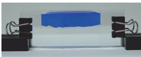
Fig. 5. Photography of the emulsion between two glasses deposited by gravity technique.
