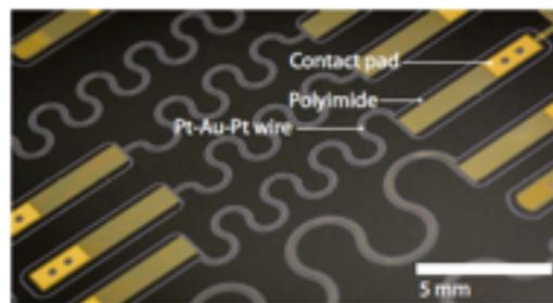
Figure 2: Photograph of the deformable thin film heaters embedded in polyimide on the handle wafer. <sup>[2]</sup>
