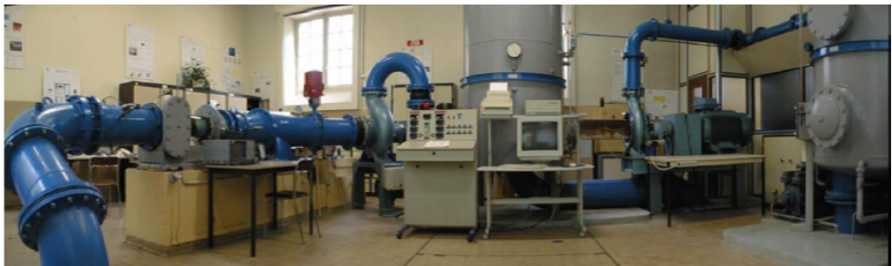
Fig. 13. Bank of experimental tests from DynFluid laboratory (Arts et Métiers ParisTech), loop of the industrial inducers
