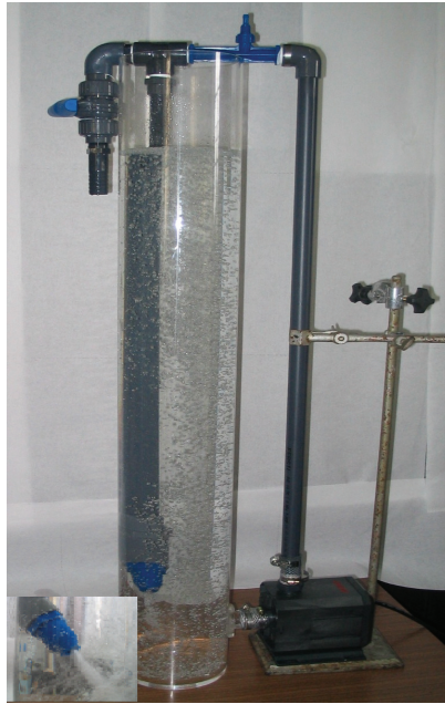
Fig. 15. The air micro-bubble bioreactor filled with clean water
