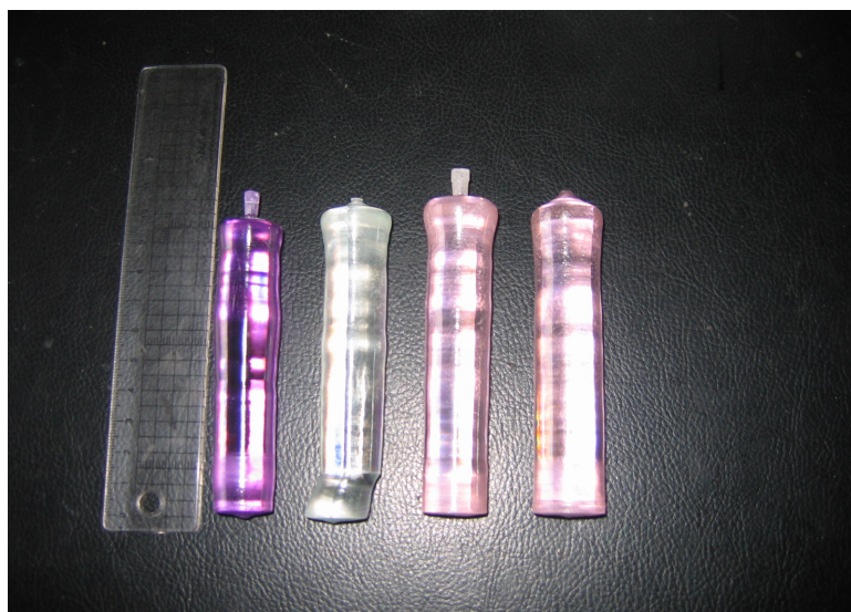
Fig. 2.4 The grown \text{Re}^{3+}:\text{NaY}(\text{WO}_4)_2 crystals ( \text{Re}=\text{Yb}, \text{Nd}, \text{Er}/\text{Yb} ).
