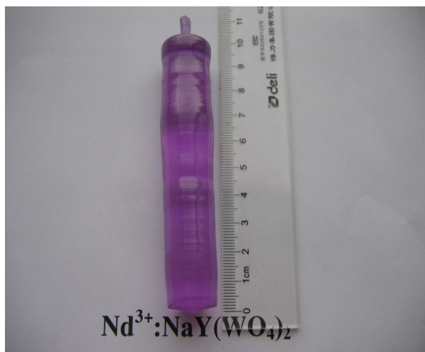
Fig. 2.2 The grown \text{Nd}^{3+}:\text{NaY}(\text{WO}_4)_2 crystal.
