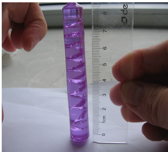
Fig. 2.1 The cracking \text{Nd}^{3+}:\text{NaY}(\text{WO}_4)_2 crystal.
