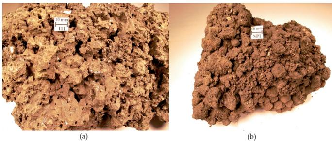
**Figure 3.** Typical macrostructures of lead sinter
