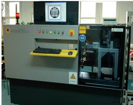
**Figure 5.** Prototypical CO<sub>2</sub>-laser sintering facility used for sintering and densification of green thin film ceramic layers.
