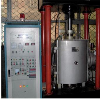
Figure 7. ZLY-60 pulse current auxiliary sintering apparatus
