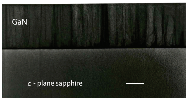
Fig. 3. MOCVD grown GaN on c -plane sapphire showing high density of threading dislocations (Selvaraj & Egawa, 2008).
