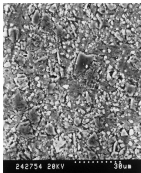
Fig. 1. Microstructure of aluminum matrix composite \text{SiC}_p/\text{A356}
