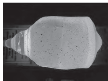
Fig.2 La-GPS single crystal grown by the CZ method.
