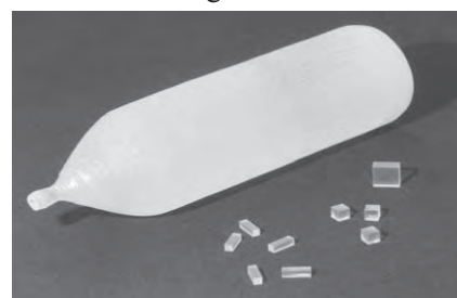
Fig.1 GAGG single crystal grown by the CZ method.
