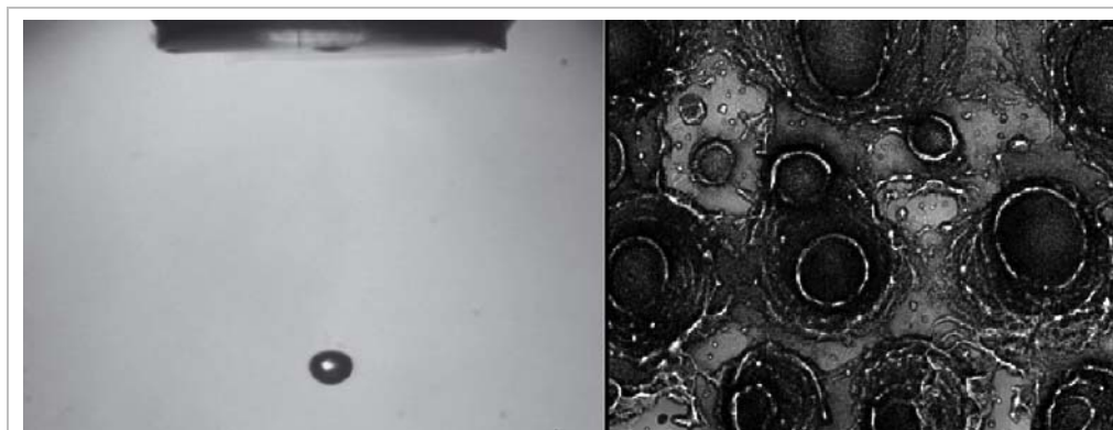
Figure 1: A typical droplet ejected by the microdrop head while approaching the substrate (left) and a magnified view of the deposition pattern (right) obtained using droplets with a diameter of 100 \mu\text{m} and a distance between centres of droplets of \sim 170 \mu\text{m} .
