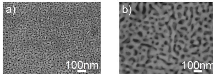
Fig. 1. SEM images of samples dealloyed in 65% conc.  $\text{HNO}_3$  for different times a) 10 min, b) 60 min. After dealloying the film consists of an irregular bi-continuous network of air pores and gold veins forming a nanoporous gold film.
