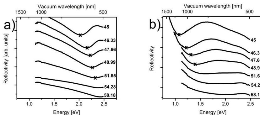
Fig. 2. p-polarised angular resolved reflectivity spectra measured in Kretschmann configuration. The value of the angle of incidence  $\theta$  in the glass is indicated on each curve. a) bulk gold film, b) nanoporous gold film. The dip in reflection shifts to shorter wavelengths with increasing angle of incidence (indicated by the crosses). This indicates the resonant excitation of propagating surface plasmons.
