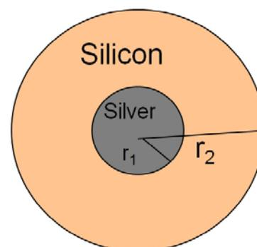
Fig. 1: A particle made of a silver core and a silicon shell
