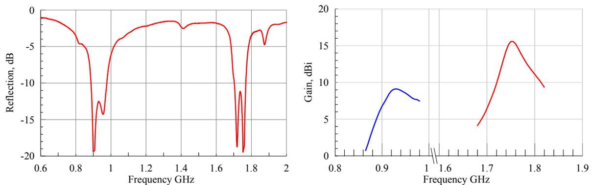
Fig. 3: Reflection response (left) and antenna gain (right) of the proposed dual-band PV-integrated antenna.
