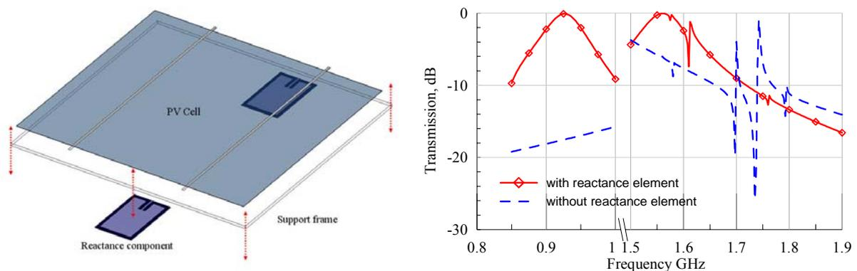
Fig. 1: Unit-cell with reactance load (left) and the transmission responses (right)
