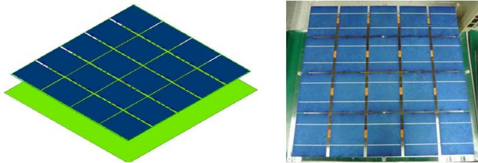
Fig. 2: The proposed dual-band PV-integrated antenna, simulation model (left) and prototype photo (right).
