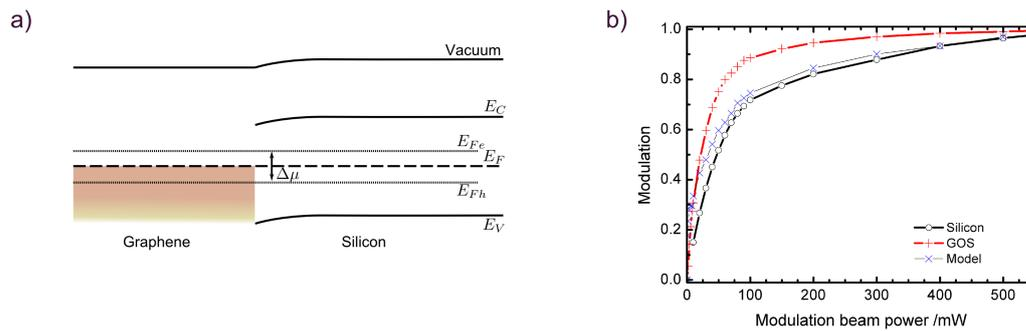
Fig. 2: a) Bandscheme of the silicon-graphene heterojunction. b) Measured dependence of the modulation depth on the modulation power for silicon and GOS. The modulation depth was averaged over a frequency band from 0.2-1.0 THz. The semi-analytic results for GOS are in good agreement.
