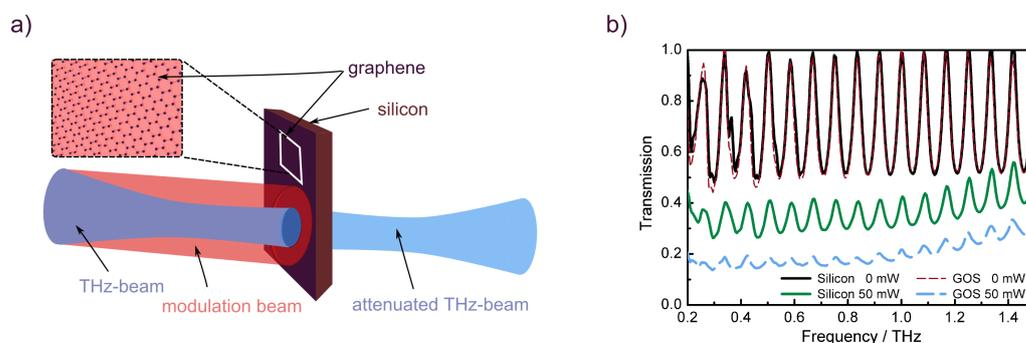
Fig. 1: (a) Schematic of the set-up for the modulation experiment. (b) Transmission spectra of the Si and GOS modulator without illumination and with an illumination power of  $P = 50$  mW.
