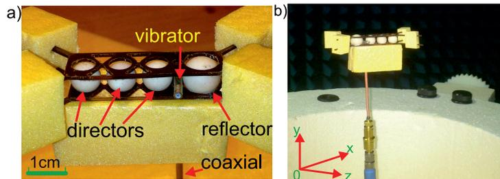
Fig. 3: Photographs of the all-dielectric Yagi-Uda microwave antenna. (a) Detailed view of the antenna placed in a holder. (b) Antenna placed in an anechoic chamber; the coordinate  $z$  is directed along the vibrator axis; the coordinate  $y$  is directed along the antenna axis.
