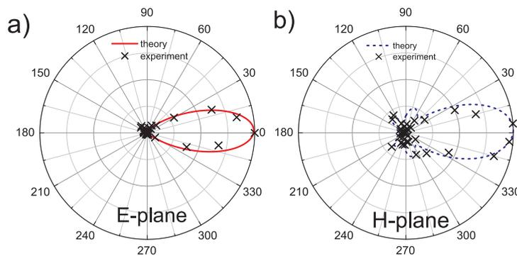
Fig. 4: Radiation pattern of the antenna in (a)  $E$ -plane and (b)  $H$ -plane at the frequency 10.7 GHz. Solid lines show the results of numerical simulations in CST; the crosses correspond to the experimental data.
