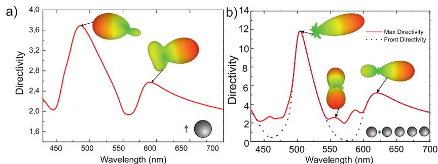
Fig. 2: (a) Dependence of the directivity  $D$  on the wavelength. (b) Directivity of the dielectric Yagi-Uda nanoantenna vs wavelength for the separation distance  $G = 70$  nm. Insert demonstrates 3D radiation pattern diagrams at particular wavelengths.
