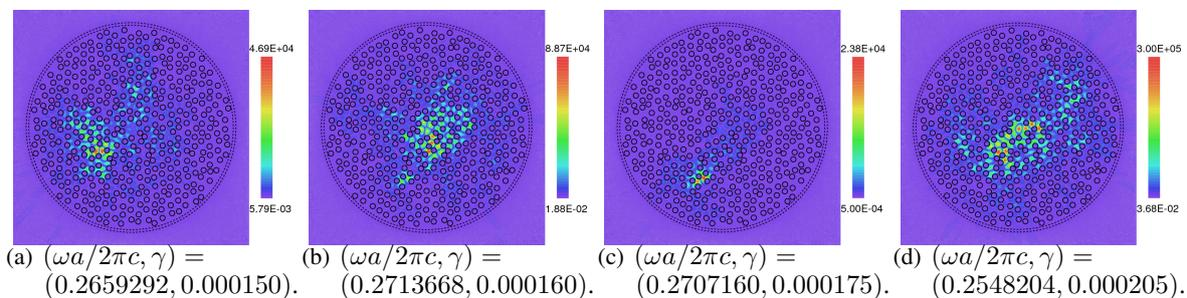
Fig. 3: Electric amplitude distributions of lasing states in a metallic disordered structure (sample 1).
