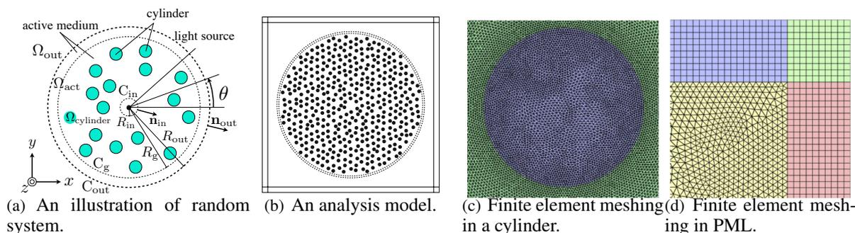
Fig. 1: Illustration, analysis model, and finite element meshing.
