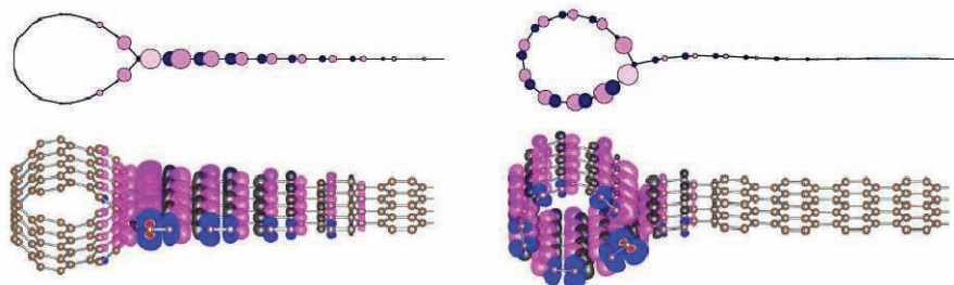
Figure 1: Structure and spin density for symmetric (left) and asymmetric (right) of nanoribbon edges terminated by armchair nanotubes. The localization of magnetization depends on the nanoribbon-nanotube junction.
