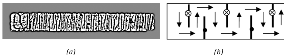
Fig.1: The labyrinth domain pattern in the beginning of the magnetization reversal of the strip: Bitter image of the structure, (a) and the sketch of the structure (b); the arrows show supposed in-plane components of magnetization direction that are separated by domain walls with perpendicular alternating up and down magnetization.
