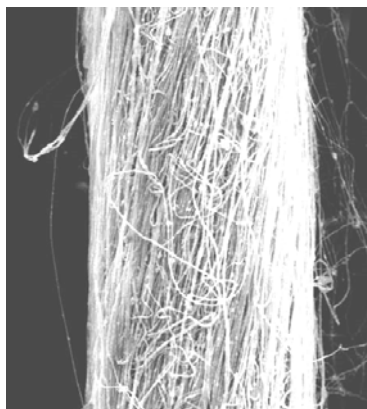
Fig.1. SEM image of obtained fiber consisting from aligned composite nanofibers.
