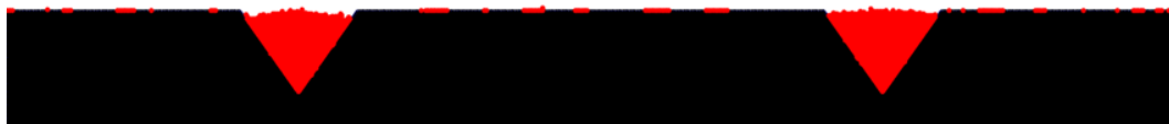
Fig. 1 – The morphology of an array of In nanostructures after deposition of 5 ML of In on an As-stabilized GaAs(001) substrate with triangular grooves with a diameter and a depth of 20 nm.
