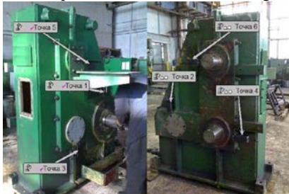
Figure 4. The scheme of the 6 points of vibration control.
