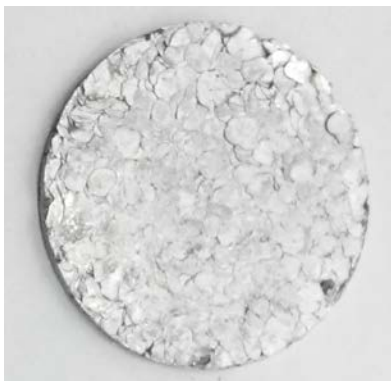
Fig. 4 Appearance of a compact made of the mechanocomposite Al + TiH_2
