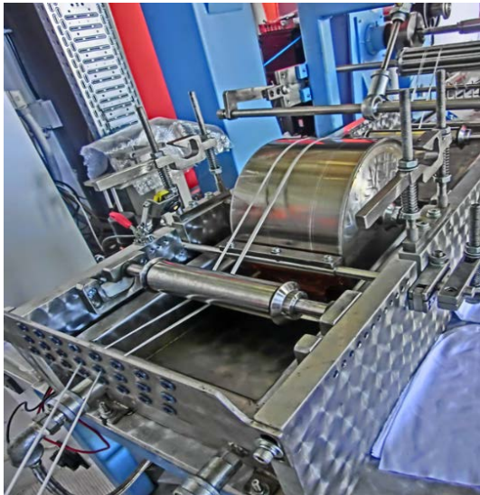
Figure 2. Filament winding machine MAW FB 6/1
