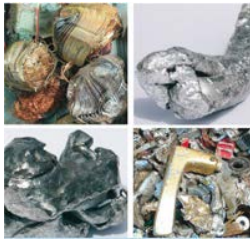
Fig. 2: Querstromzspanner's results. There are inclusions and compactions of the metal component cover. (6)
