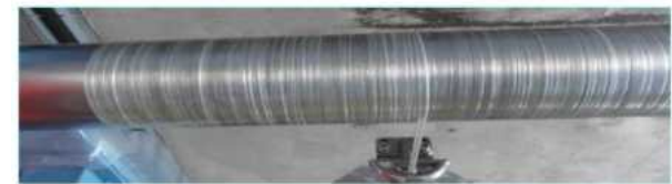
hoop winding ( \theta = 90^\circ )
