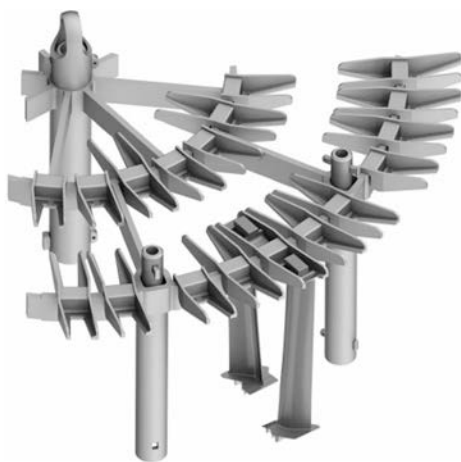
Fig. 4. Increased capacity of the equipment shown in Fig. 3a by the use of double hook [9]
