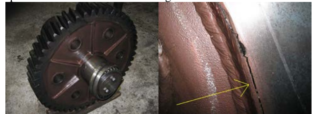
Figure 6. The photo of the real welded gearwheel, with the cracks. As can be seen, due to this method, was sufficiently prevented a serious accident and were spared a lot of resources.
