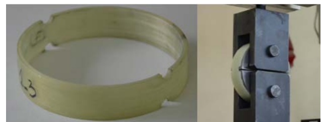
Figure 4. Split-disk test specimen and test fixture with specimen for hoop tensile testing
