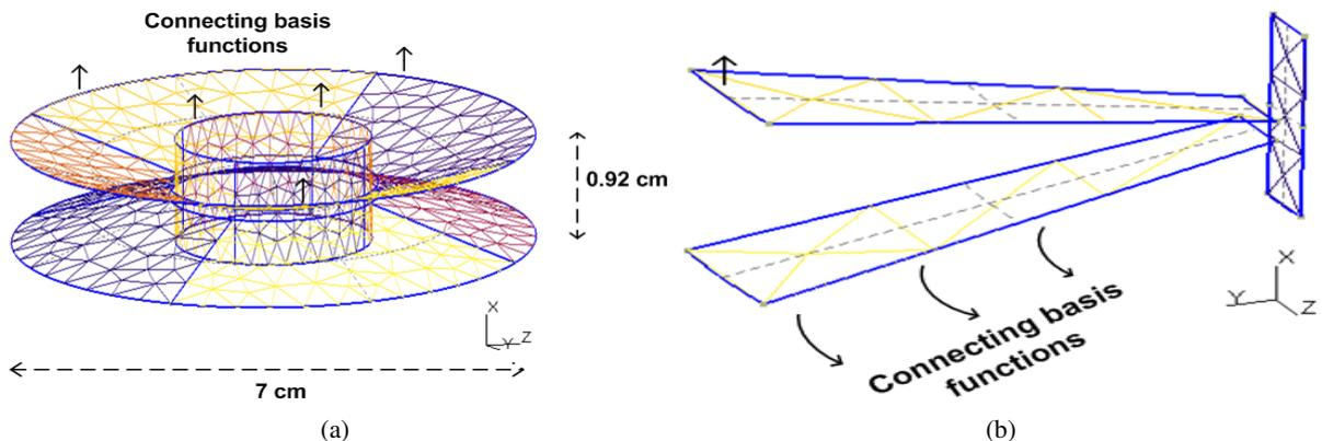
Fig. 1: Mesh of the cloak (a) full cloak with cylinder (b) a sector of the cloak and cylinder
