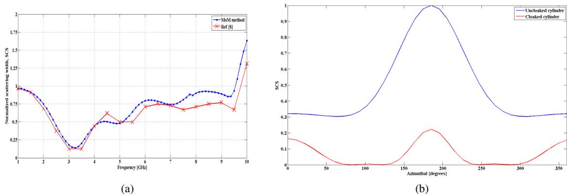
Fig. 2: (a) SCS of the cloaked cylinder normalized to the uncloaked cylinder over frequency compared to [8] (b) SCS of the cloaked and uncloaked cylinder at 3.25 GHz over azimuthal.
