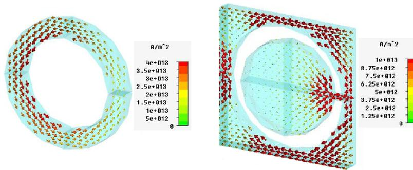
Fig. 3: Electric currents over the SRR and the C-SRR at their resonant frequencies for the case of the smallest resonators with radius  $r = 50\text{nm}$ .
