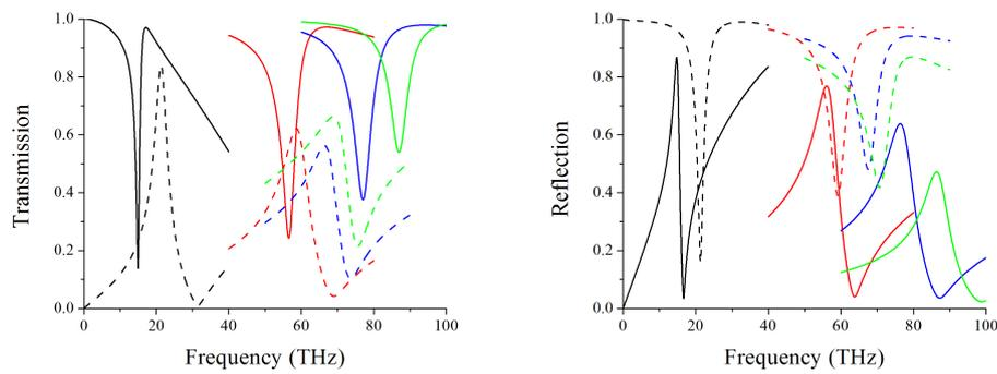
Fig. 2: Scattering parameters for metasurfaces of SRRs (solid lines) and C-SRRs (dashed lines). The inverse radius expressed in  $\mu\text{m}^{-1}$  are  $r^{-1} = 1$  (black), 5 (red), 10 (blue), and 20 (green).
