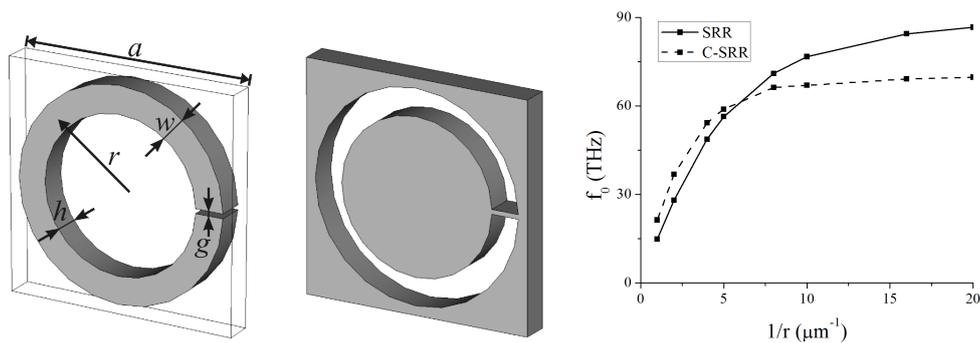
Fig. 1: From left to right, unit cells for metasurfaces made of SRRs and C-SRRs, and plot of resonant frequency versus the inverse radius for both metasurfaces.
