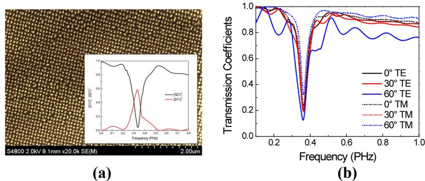
Fig. 3 (a) SEM picture of a Metaflex composed of gold disks (period 100 nm, diameter 70 nm). The inset shows the calculated reflection (red) and transmission (black) vs frequency. (b) Simulated transmission spectra for different incidence angles.
