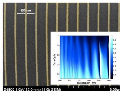
Fig. 2: SEM picture of a one-dimensional grating (period 1 μm and wires width 150 nm). The inset shows the calculated transmission vs wavelength for different duty cycles.
