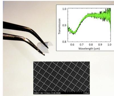
Fig. 1: A metaflex sample held with tweezers. The bottom inset shows a SEM picture of a fishnet structure, the top inset shows its transmission curves for orthogonal polarizations, aligned along the wires.
