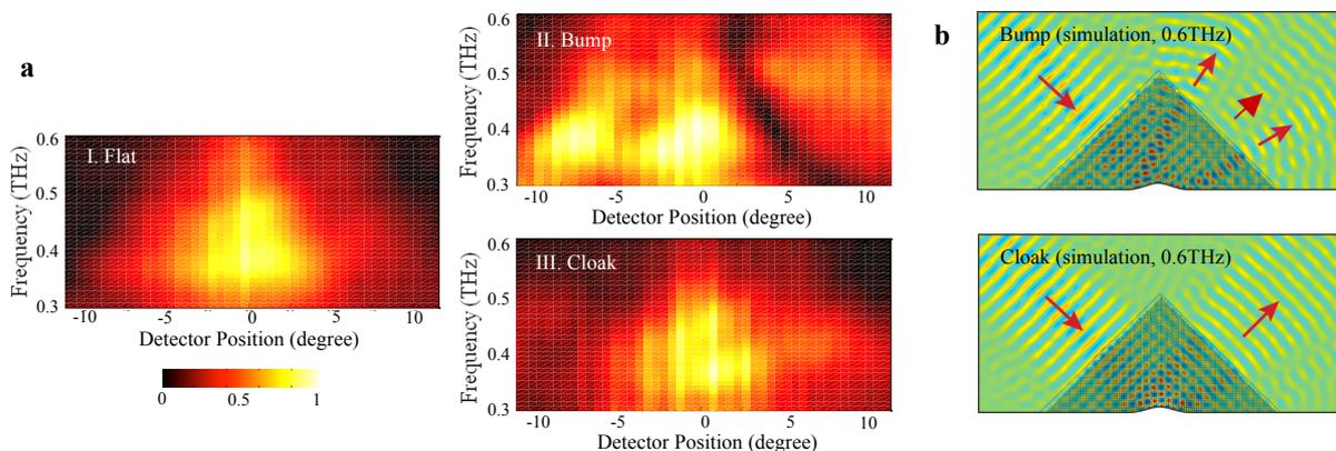
Fig. 2: a, Reflection measurement results for case I. flat metal surface, case II. bump, and case III. cloak. b, Simulation results for case II and case III at 0.6 THz.
