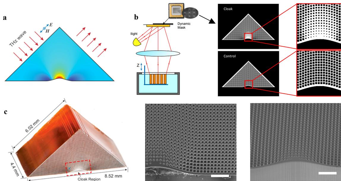
Fig. 1: Fabrication and characterization of 3D THz cloak. a, 2D spatial refractive index distribution of the cloak structure for TM polarized THz wave. b, Schematic diagram illustrating projection micro-stereolithography system being used to fabricate 3D cloaking device and the mask design for cloak sample and control sample. c, Optical and SEM images of fabricated cloaking device. Bar: 500  $\mu\text{m}$ .
