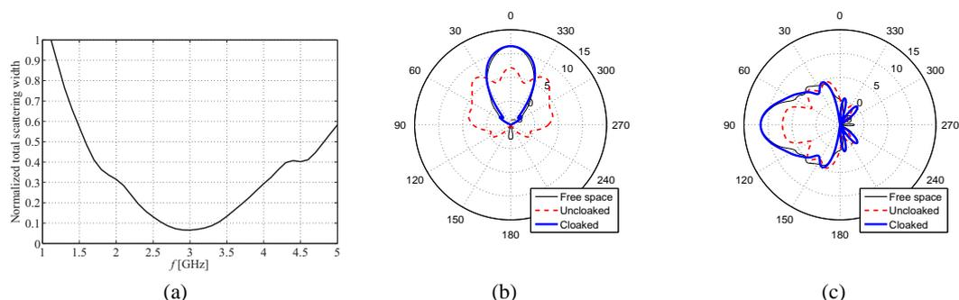
Fig. 2: Simulation results: (a) Scattering width for an infinitely high cloak; (b) Simulated directivity of the horn antenna in the  $xy$ -plane ( $f = 3$  GHz); (c) Simulated directivity of the horn in the  $xz$ -plane ( $f = 3$  GHz).
