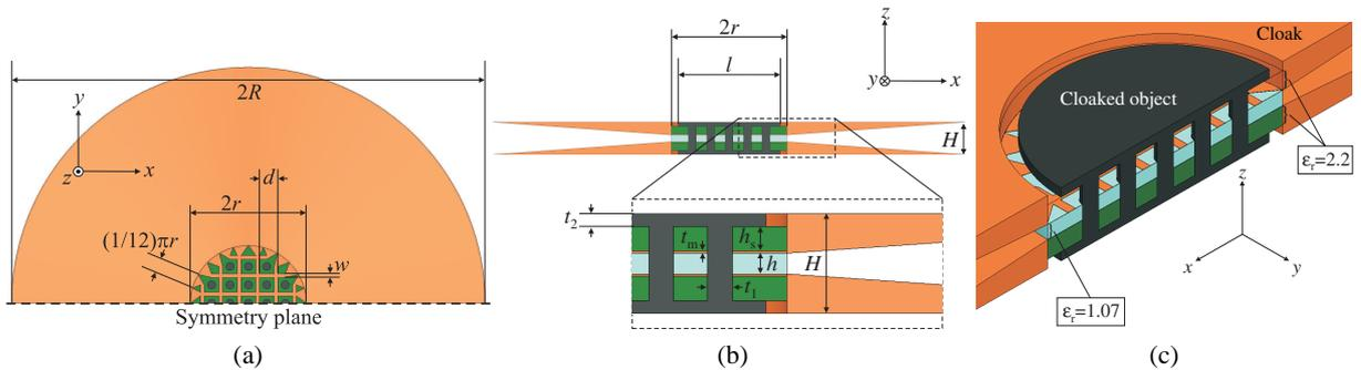
Fig. 1: Cloak geometry for one half of a single cloak layer: (a) xy-plane view (b) xz-plane view (c) cut along xz-symmetry plane (upper substrate invisible).
