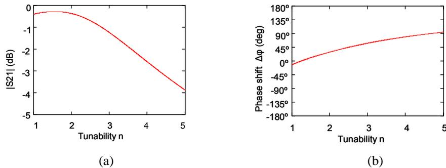
Fig. 2: Transmission coefficient (a) and phase shift (b) versus tunability  $n$  for a single cell of a CRHL TL.
