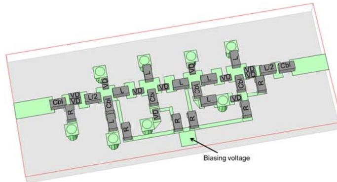
Fig. 3: Layout of the four-cell  $0^{\circ}$ - $180^{\circ}$  CRLH TL phase shifter.
