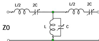
Fig.1: Equivalent diagram of a symmetric unit cell of composite right/left handed transmission line.
