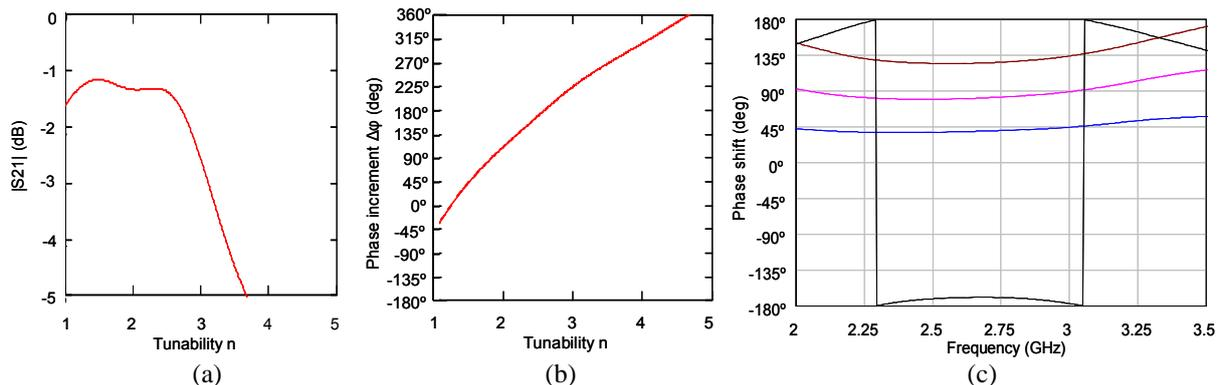
Fig. 4: Insertion loss (a) and phase increment (b) versus tunability; panel (c) displays the frequency dependence of  $180^{\circ}$ ,  $135^{\circ}$ ,  $90^{\circ}$ , and  $45^{\circ}$  phase shifts of the 4-cell CRLH TL phase shifter.
