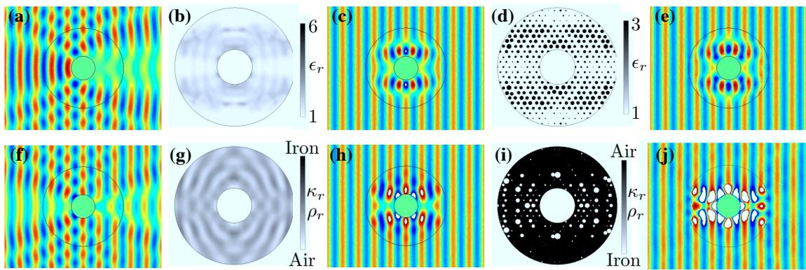
Fig. 1: The cloak designs and FE simulations for an  $E_z$  polarized wave (a)-(e) and an acoustic wave (f)-(j). (a) and (f) show the non-cloaked cylinders. (b), (c), (g) and (h) show the graded designs and resulting fields. (d), (e), (i) and (j) show the designs obtained using MMOS and resulting fields.
