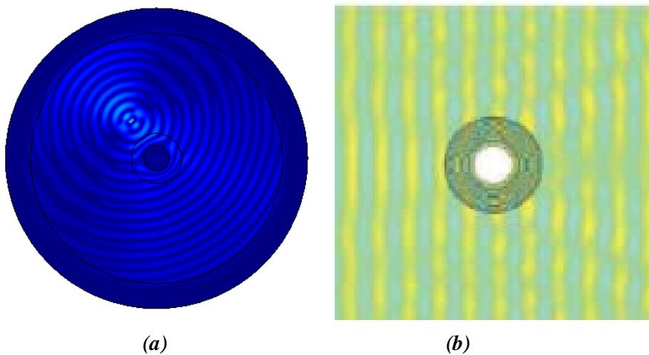
Fig. 1 (a) Magnitude of the in-plane displacement field for an elastic cloak achieving the control of coupled pressure and shear waves in presence of a point force. (b) Out-of-plane displacement field for a multi-layered elastic cloak achieving the control of bending waves over a large bandwidth.
