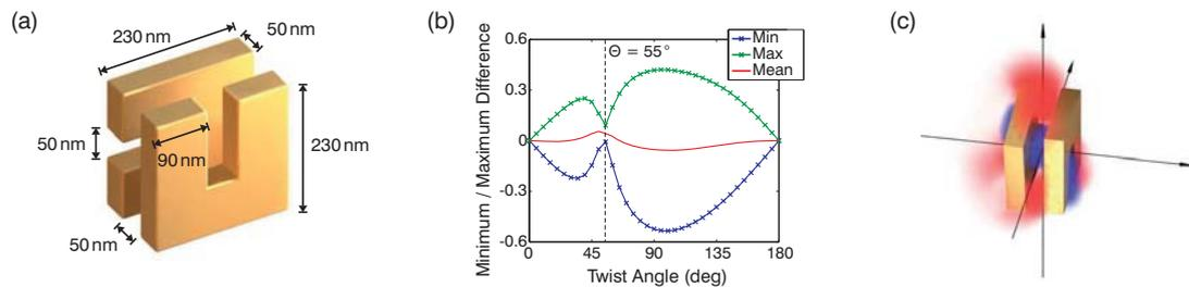
Fig. 2: Chiroptical response of the stereometamaterial. (a) Dimensions of the structure. (b) Extreme values of the transmittance difference between left- and right-handed circularly polarized light for different twist angles  $\Theta$ . For  $\Theta = 55^\circ$  one finds a non-trivial scenario with minimum chiroptical response. (c) Enhanced chirality change for  $\Theta = 110^\circ$  (angle with maximum chiroptical response).
