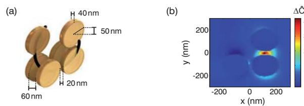
Fig. 3: (a) Plasmonic gold oligomer with helix-like geometrical chirality. (b) Slice through the chirality change map perpendicular to the propagation direction of the incident light at  $z = -38$  nm. The metamaterial shows an enhancement of more than a factor of 40.
