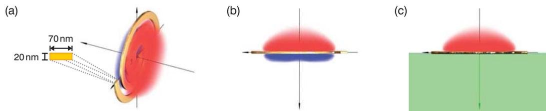
Fig. 1: Distribution of enhanced chirality change  $\Delta\hat{C}$  caused by a planar gold spiral. (a) Perspective view. (b) Side view showing the clear separation between regions where the handedness of the incident light is preserved (red) or changed (blue). (c) Only one of these regions can be accessed in presence of a substrate.
