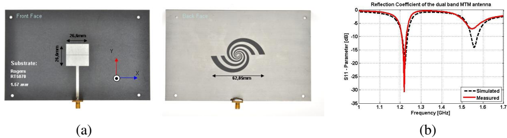
Fig. 1: Dual-Band MTM antenna: a) Front and Back faces. b) Reflection parameter ( S_{11} )
