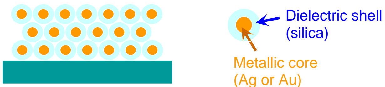
Fig 1: Schematic view of a regular assembly of core-shell nanoparticles. The metal cores are separated by twice the thickness of the dielectric shell (Silica).
