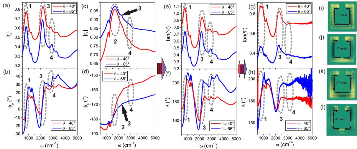
Fig. 2: The incident plane is parallel to the gap. Amplitudes (a), (c) and the phases (b), (d) of the reflection coefficients for p- and s-polarizations, respectively at two different angles of incidence are shown. Calculated (e), (f) and measured (g), (h) ellipsometric spectra are presented. The distribution of the perpendicular component of the surface electric field and current density for (i) first, (j) second, (k) third and (l) fourth plasmonic modes.
