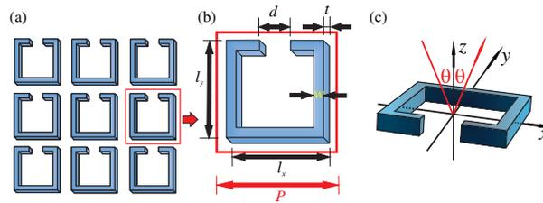
Fig. 1: (a) The part of the periodic structure and (b) unit cell are shown. (c) The incident plane ( $xz$ ) is parallel to the gap.
