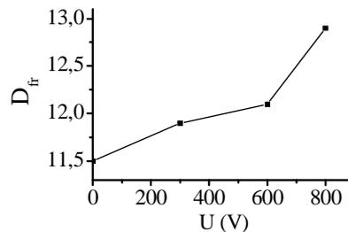
Fig. 3: Dependence of fractal dimension on bias voltage.
