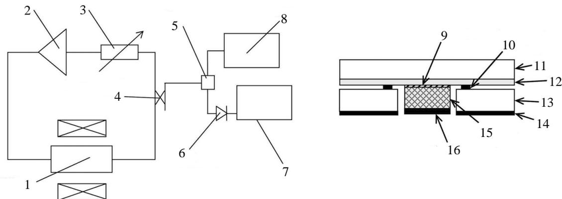
Fig. 1: Schematic diagram of the active resonance ring (left), ferrite-ferroelectric delay line (right). 1 - delay line, 2 - microwave amplifier, 3 - tunable attenuator, 4 - directional coupler, 5 - splitter, 6 - detector, 7 - oscilloscope, 8 - spectrum analyzer, 9 - upper electrode, 10 - microstrip antennae, 11 - GGG, 12 - YIG, 13 - substrate, 14 - metallization, 15 - ferroelectric layer, 16 - bottom electrode.
